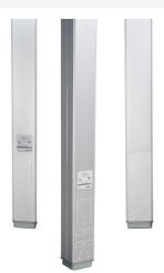
Two-compartment pole. Nominal material thickness .050" [1.8mm]. Length: 15' 5" [4.7m]. Furnished unwired without outlets. Two 8" [203mm] removable covers with KOs for modular jacks and modular furniture communication outlets. Mounting hardware, entrance end plate and ceiling trim plates furnished. NOTE: Custom options - features such as colors or other lengths [20' [6.1m] maximum] available on custom orders.
