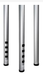
Satin anodized extruded aluminum pole. Nominal material thickness .060" (1.5mm). Length: 10' 5" (3.2m). Two-compartment (power and communication channels). Factory wired with four 15A 125V NEMA 5-15R devices. Provided with one 1/2" (12.7mm) trade size K0 in cover at base for communications. T-bar mounting hardware, ceiling trim kit, and feed box furnished. NOTE: There is no method provided for mounting data in this pole.
