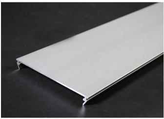
6063-T5 extruded aluminum, satin anodized finish, .075'' (1.9mm) wall thickness. This cover is packed eight 5' (1.5m) lengths per carton. Made in U.S.A.
