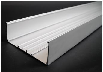
6063-T5 extruded aluminum, satin anodized finish, .080'' (2.03mm) wall thickness. Base has four ribs for snap-in divider. AL200B-10 is packed four 10' (3m) lengths per carton. Made in U.S.A.
