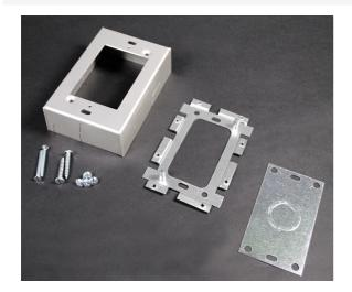
Single Gang Shallow Device Box. Designed for standard shallow switches and receptacles. Base has open back plate for mounting to existing wall box and solid black plate insert with 1/2" and 3/4" trade size Kos to close opening.
