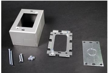
Single Gang Deep Device Box. For larger receptacles and deep devices such as those of signal and alarm systems. Base has open black plate for mounting to existing wall box and solid black plate insert with 1/2" and 3/4" trade size Kos to close opening. Accepts industry standard faceplates for communication devices. Aluminum
