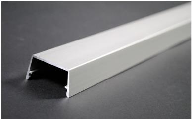
1 7/16" (37mm) wide, 6063-T5 extruded aluminum, satin anodized finish, .60" (1.5mm) nominal thickness. Cover packed (12) 5' (1.5m) lengths per carton.
