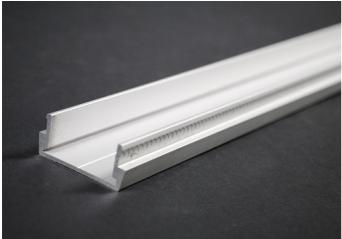
1 7/16" (37mm) wide, 6063-T5 extruded aluminum, satin anodized finish, .60" (1.5mm) nominal thickness. Base packed (12) 5' (1.5m) lengths per carton.
