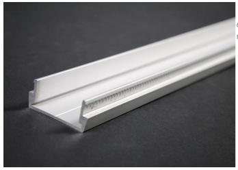
6063-T5 extruded aluminum, satin anodized finish, .60" (1.5mm) nominal thickness. Packed six 10' (3m) lengths per carton.
