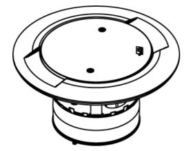
Complete plug assembly for abandoning an open 4" (102mm) diameter hole. Assembly includes intumescent fire-stop material to maintain the fire-classification of the floor, integral retainer ring to prevent the unit from pulling up through the floor, and a black diecast aluminum cover.
