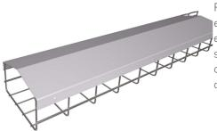
Stainless steel snap on peak cover for wire mesh tray 316L, 4"" width. Food and beverage processing plants are often harsh, challenging environments that demand extra consideration when it comes to equipment. With frequent washdowns and exposure to chemicals, stainless steel options are ideal due to their durability and resistance to corrosion. Stainless steel cable tray and accessories are easy to install, clean and meet National Sanitation Foundation standards.
