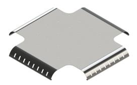
Junction bridges keep cables separated at tees and crosses in Cablofil cable management for optimum network signal integrity. The unique design creates smooth cable transitions to keep cables from kinking and bunching. Bridges mount in place using a BC1 Bridge Clip bolted to CE35 or EZT90/RADT90 junction hardware. Each bridge is predrilled with BH75 Bridge horn mounting holes and slots to secure cables with nylon zip ties.
