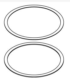
Used for floor coverings greater than 5/16" (7.9mm). This tile shim will allow the top surface of the cover to be flush with the finished floor. Includes six (6) 1/16" (1.6mm) thick shims. Up to a total of 3/8" (9.5mm) of adjustment.
