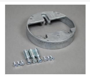
Adjusting ring (with three adjusting screws) for use with 437 Attaching Rings - communication only (brass and polycarbonate fittings) and power for polycarbonate fitting only. 3 25/32" (96mm) 0.D.
