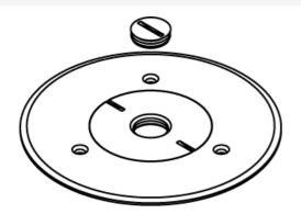
Brass cover plate with 1/2" (12.7mm) threaded opening 5 1/2" (140mm) for carpet. NOTE: For carpet or tile installations. All cover plates are furnished with gasket and three screws. The 895P Polycarbonate Series Cover Plates must be field modified for dual service.
