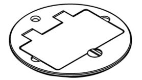
Brushed aluminum GFI receptacle cover plate, 4 1/4" (108mm) for tile. NOTE: For carpet or tile installations. All cover plates are furnished with gasket and three screws. The 895P Polycarbonate Series Cover Plates must be field modified for dual service.
