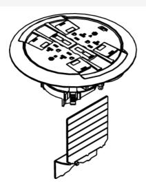
For 881PVC Floor Box. Kit complete with two (2) 20A duplex receptacles, (receptacles can be wired as standard or Isolated Ground), flange and slide holder, 881ADP Adapter, and 881DIV Divider. Provided with Wiremold CM Series Open System unloaded adapters, Ortronics Series II and TracJack adapters. Modular jacks sold separately. CAUTION: Not for use on concrete pours less than 4 1/2" (114mm) deep. Not for use when concrete is the finished floor. Use only for tile, carpet, or wood covered floors.
