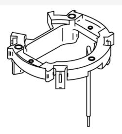
Used to attach wiring devices and cover plates to PVC box. Locks into place without using glue or mechanical fasteners. Compensates for up to 10° of tilt if box is not level. Ground wire is factory attached to the adjusting ring. One ring required per box, single- or dual-service, ordered separately.
