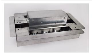
3-Gang Fire Classified Steel Floor Box. Adjustment range over deck of 2" (51mm) minimum to 6-1/2" (165mm) maximum. One 1 1/4" (32mm)and two 2" (51mm) conduit feed openings. Inside Gange Capacity - 67.5 cubic inches. Outside Gang Capacity - 54 cubic inches each gang. This floor box preserves up to a 3- hour fire rating of floors in which it has been installed.
