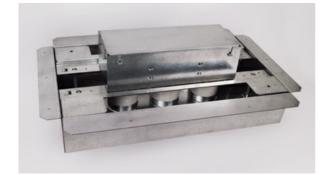
3-Gang Fire Classified Steel Floor Box. Adjustment range over deck of 2" (51mm) minimum to 6-1/2" (165mm) maximum. One 1 1/4" (32mm)and two 2" (51mm) conduit feed openings. Inside Gange Capacity - 67.5 cubic inches. Outside Gang Capacity - 54 cubic inches each gang. This floor box preserves up to a 3- hour fire rating of floors in which it has been installed.
