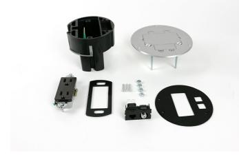
Includes round PVC floor box, one 15A, 125V tamper-resistant decorator style duplex receptacle, one coax F connector, one RJ45 Category 5e connector, and brushed aluminum duplex opening cover plate with single flip lid.
