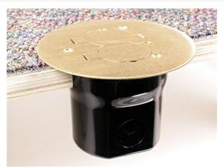
Includes 862 Series Floor Box, one 15A, 125V tamper-resistant brown duplex receptacle, and one 895 brass duplex receptacle cover for carpet. Order 862KIT when using in concrete floor.
