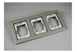
Three-gang powder-coated aluminum combination carpet and tile flange, 6.080'' x 13.17'' (154.4mm x 335mm). Accepts Ortronics MAB6TJ TracJack and MAB3S2 Series II adapters and Wiremold CM Series inserts, sold separately. NOTE: Brass covers and flanges are not interchangeable with aluminum or nonmetallic covers and flanges. Nonmetallic covers are interchangeable with aluminum flanges.
