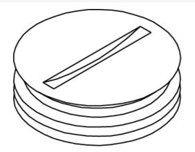
3/4" (19.1mm) diameter brass abandon plug. Thread size is pipe thread size.
