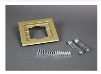
One-gang powder-coated aluminum combination carpet and tile flange, 6" x 5" (152.4mm x 127mm). Accepts Ortronics MAB6TJ TracJack and MAB3S2 Series II adapters and Wiremold CM Series Open System inserts, sold separately. NOTE: UL Listed for tile, terrazzo, and carpet floors. Brass covers and flanges are not interchangeable with aluminum or nonmetallic covers and flanges. Nonmetallic covers are interchangeable with aluminum flanges.
