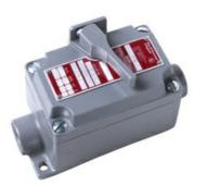
Double-Pole, Single Phase Switch in a NEMA 7 and 9 Enclosure for Hazardous Locations. Class I - Groups C, D Class II - Groups E, F, G. 30A, 600Vs. Slotted opening on enclosures allows for lock-out, tagout functionality.
