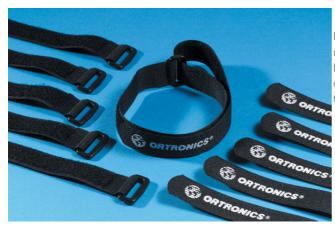
D-ring cable management straps provide an organized solution for the management of horizontal distribution cables. The 3/4" wide straps have a hook and loop type closure to secure and administer cables without damaging the construction of the copper or fiber cable. Sold in packages of ten. Black.
