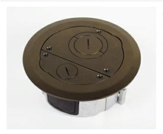
The new FloorSource Series Round Furniture Feed Floor Box is designed to work in both wood and raised floor applications, perfect for feeding power and data to modular furniture. Constructed of die cast aluminum material, the furniture feed floor box can be divided for dual service. Each 3 inch (76mm) tall box is provided with a durable sheet metal cover. This box accepts the 6 inch (182mm) round Evolution Series furniture feed covers.
