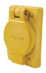
Turnlok Watertight Single Receptacle, 30amp 3 250 volt, NEMA Configuration L15-30, Impact resistant Valox lid, cover plate, and receptacle body withstand impacts, chemical, and corrosion.
