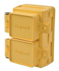
Turnlok Watertight Duplex Receptacle, 15amp 277volt, NEMA Configuration L7-15, Impact resistant Valox lid, cover plate, and receptacle body withstand impacts, chemical, and corrosion.
