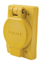
Straight Blade Watertight Single Receptacle, 20amp 250volt, NEMA Configuration 6-20, Impact resistant Valox lid, cover plate, and receptacle body withstand impacts, chemical, and corrosion.
