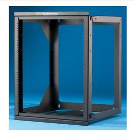
Legrand swing wall mount racks offer the flexibility of an 18 in deep wall mounted unit for mounting telecommunications and data equipment. They are available in three heights, with front swing gates and 19 in #12-24 threaded EIA pattern. Black.
