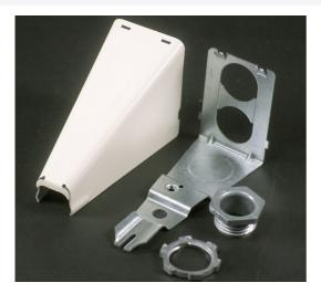
Eliminates need to offset raceway when connecting to surface type panel boxes. Adjustment from surface to center of bushings is 5/8" (15.9mm) minimum to 1 3/8" (35mm) maximum. When used as adjustable offset connector, break out metal between the two holes. When used with 700 Series Raceway, break out crescent twistout in cover. 1/2" trade size chase nipple and HICknut furnished.
