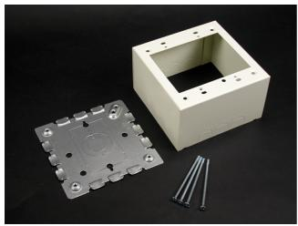
Designed especially for use in the installation of signal system and alarm wiring. Base has 1/2" trade size KOs. Larger gang boxes available by special order. Two-gang: 4 3/4" L x 4 3/4" W (121mm x 121mm). Accepts NEMA double-gang standard faceplates. NOTE: Certified to Canadian Safety Standards for sale in Canada. When ordering these products, change the "V" color prefix to "vc" or the "WH" color suffix to "WHC" to denote the Canadian versions.
