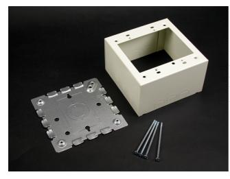
For deep devices such as momentary contact, remote control switches, and hospital signaling system devices. Base has 1/2'' trade size KOs. Larger gang boxes available by special order. Twogang: 4 3/4'' L x 4 3/4'' W (121mm x 121mm). Accepts NEMA doublegang standard faceplates. NOTE: Certified to Canadian Safety Standards for sale in Canada. When ordering these products, change the ''V'' color prefix to ''vc'' or the ''WH'' color suffix to ''WHC'' to denote the Canadian versions.
