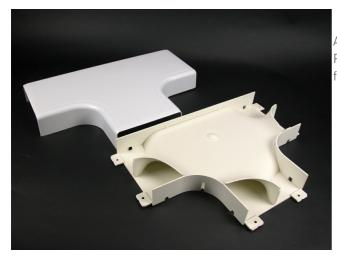
A full capacity tee fitting for branching raceway at right angles. Provides separation of services and 2'' (51mm) cable bend radius for UTP and Fiber Optic installations.
