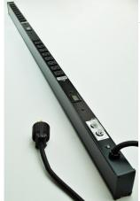
Two circuits with two 20A resettable circuit breakers and two lighted LCD digital ammeters. Eighteen 20A outlets with T-slots, black housing. 12' (3.6m) cord. Length 54" (1.4m).
