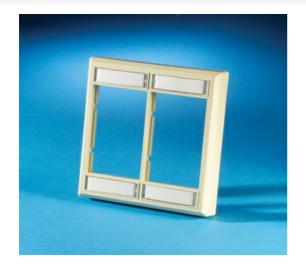
Series II Double Gang Faceplate accepts a wide variety of Series II modules. This low profile plate provides six units of module space and is .75" deep.
