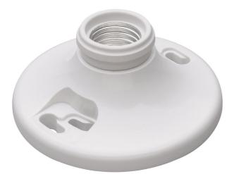
Medium base, phenolic, one-piece keyless, 4 terminals with Tamper-Resistant-drive screws, fits 3 1/4-inch and 4-inch boxes, with cage neck.
