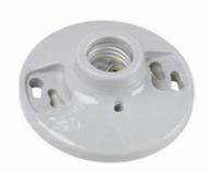
Medium base, porcelain, one piece keyless, 4 terminals with Tamper-Resistant-drive screws, fits 3 1/4-inch and 4-inch boxes.
