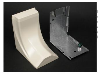
Eliminates need to offset 2400 Series Raceway when connecting with surface panel boxes. Has 3/4'' and 1'' concentric trade size KOs with 1'' trade size KO elongated so adjustment from surface to center of bushing is 1'' (25mm) minimum to 1 5/8'' (41mm) maximum. Has twistouts for transition to 1500 and 2600 Pancake Raceways.
