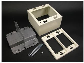
Divided, two-gang, labor saving, over-the-raceway device box. Allows both power and low voltage at a single point-of-use. Accepts 5507 Series Faceplates, Ortronics TracJack and Series II Modules (requires S2-EPL Plate), Pass and Seymour Activate Series Inserts (requires CM-EPLA Plate), and Wiremold Open System Communication Modules (requires CM-EPLA Plate).
