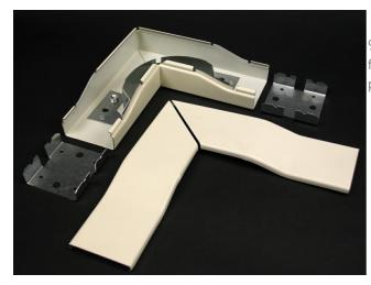
90 degree flat corner elbow provides 2'' (51mm) cable bend radius for fiber optic and UTP/STP cable installations. Ideal for lay-in or pull-through installations. Couplings included.
