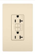
Conducts an automatic test every three seconds, ensuring it's always ready to protect. If the device fails the test, the indicator light flashes to signal that the GFCI should be replaced. It also has our proven SafeLock<sup>TM</sup> Protection feature: if critical components are damaged and protection is lost, power to the receptacle is disconnected. For more detailed information, visit our GFCI Outlets and Receptacles page.
