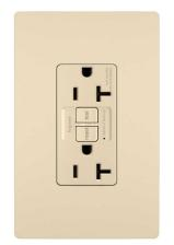
Conducts an automatic test every three seconds, ensuring it's always ready to protect. If the device fails the test, the indicator light flashes to signal that the GFCI should be replaced. It also has our proven SafeLock<sup>™</sup> Protection feature: if critical components are damaged and protection is lost, power to the receptacle is disconnected. For more detailed information, visit our <u>GFCI Outlets and Receptacles</u> page.
