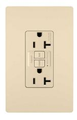
Conducts an automatic test every three seconds, ensuring it's always ready to protect. If the device fails the test, the indicator light flashes to signal that the GFCI should be replaced. It also has our proven SafeLock<sup>TM</sup> Protection feature: if critical components are damaged and protection is lost, power to the receptacle is disconnected. For more detailed information, visit our <u>GFCI Outlets and Receptacles</u> page.
