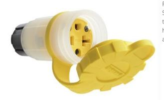
Rated watertight for 1,500 psi high-pressure hosedown, Pass and Seymour watertight GCM plugs and connectors feature multiple seals to ensure protection against the environment. The transparent body houses dual LED lights with 360 visibility, indicating ground continuity and power status, while providing a NEMA 6P/IP67 rating.
