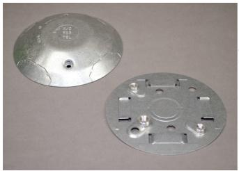
May be used as a cross, tee or elbow. Cover has 1/2" trade size KO. Base has 1/2" and 3/4" concentric trade size KOs to enable connection to floor outlet boxes or underfloor duct systems (use Chase nipple not included). Two 1500WC Wire Clips included.
